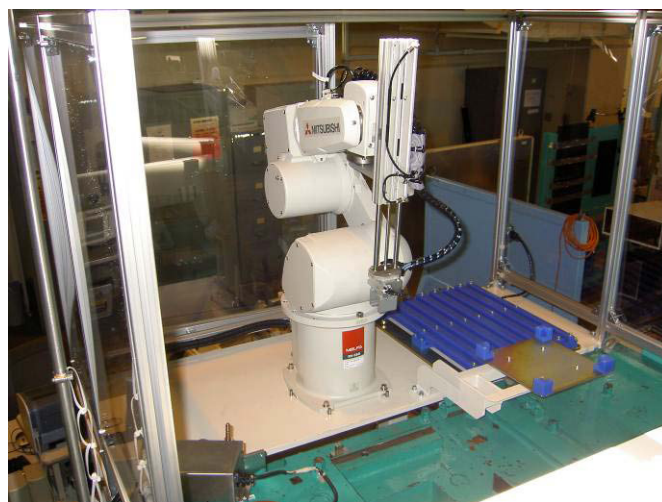
Fig.1 A revolute joint robot of the automatic PGA system
