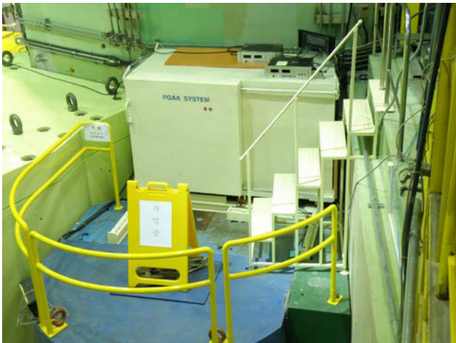
Figure 1. Thermal neutron PGAA (SNU-KAERI) facility at the ST1 horizontal beam line of the HANARO research reactor.
