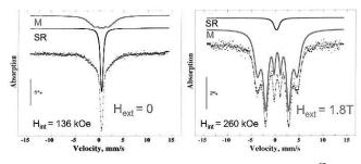
Figure 3. Mössbauer spectra of single crystal  $La_{0.9}Ca_{0.1}Mn(^{57}Co)O_3$  at T=175K.
