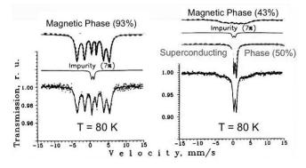
Figure 2. Mössbauer spectra of as prepared and deoxygenated  $Nd_{2-x}Ce_xCu(^{57}Co)O_4$ .
