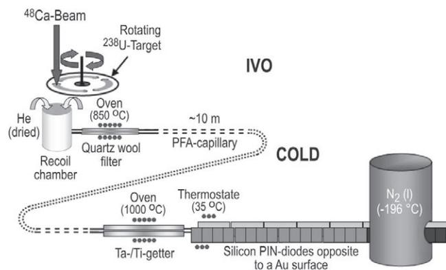
**Figure 2.** Schematic view of the experimental set up used in the first experiment on element 112 at the GSI. The upper left part depicts the In-situ Volatilization (IVO) part attached to the rotating target wheel. It is coupled to the Cryo On-Line Detector (COLD) with its Si PIN-diodes monitoring the opposite Au-coated side of the thermochromatographic channel. Figure from Reference 1.
